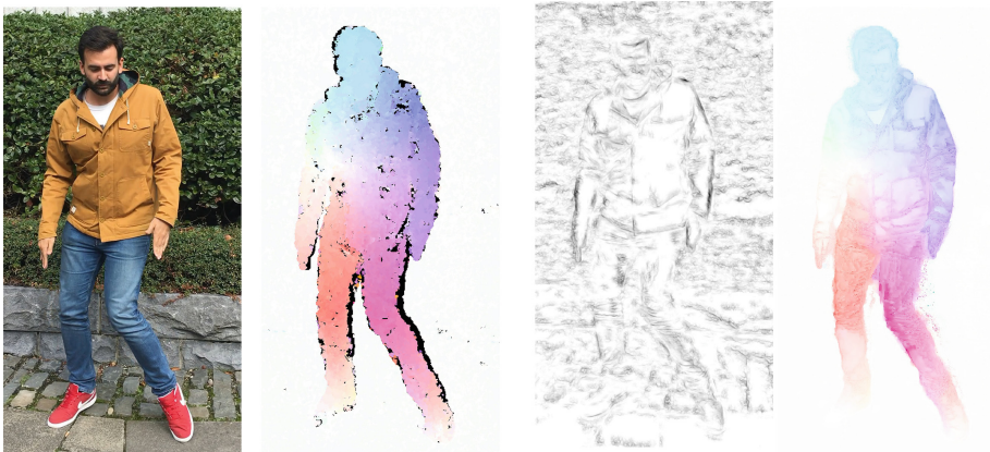
Fig. 3. From left to right, dense optical flow calculation: For a particular viewpoint, the input RGB image, (1) nearest neighbour field estimate from CPM, (2) SED detected edges, (3) interpolated dense STEA output. Conventional colour coding has been used to illustrate the orientation and intensity of the optical flow vectors. Orientation is indicated by means of hue while vector magnitude is proportional to the saturation i.e. negligible motion is represented by white, high-speed motion is shown in highly saturated color [24].
